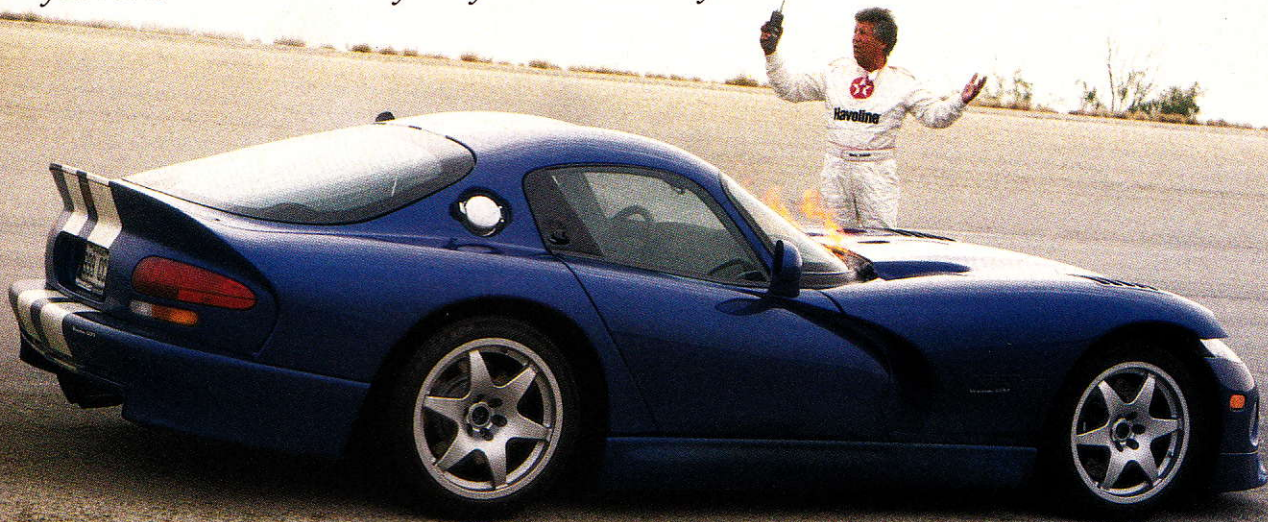
■ Mario waits helplessly as the Venom 600 catches fire, the result of a burst oil line that ended an impressive 205.4-mph run.
